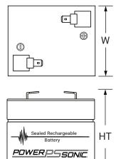
2.00 (51) W: 1.65 (42) 2.00 (51) H: HT: 2.20 (56) Tolerances are +/- 0.04 in (+/- 1mm) and +/- 0.08 in. (+/- 2mm) for height dimensions. All data subject to change without notice.
